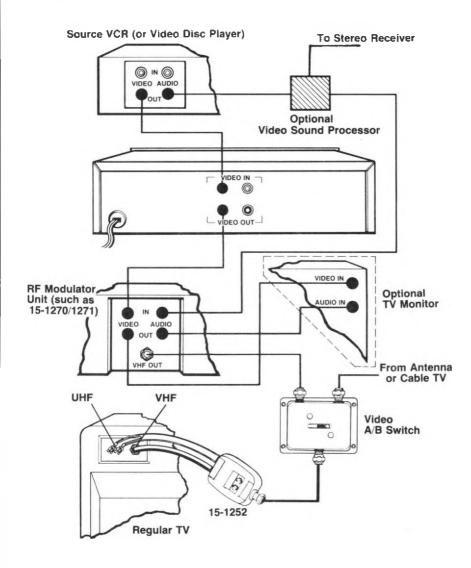
**Note:** If you use a regular TV for viewing, the A/B switch will give you easy access to cable or antenna TV broadcasts.
