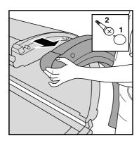
Unscrew the body cooling fan on the left side of the canopy and take it out.
