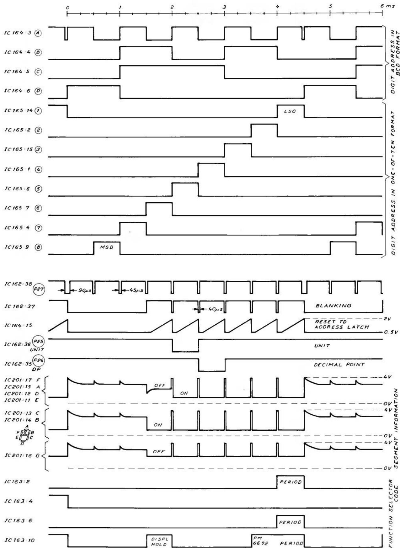
Fig. 2.13 Timing diagrams for Microcomputer - Display - Function Selector communication.
