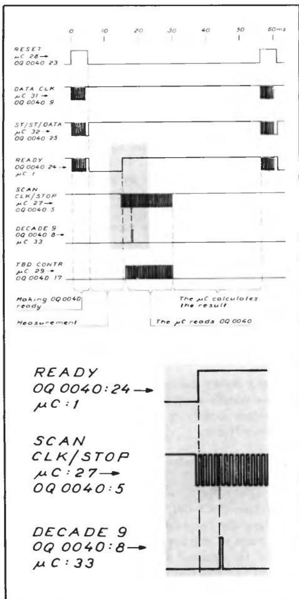
Fig. 2.11 Timing diagrams for microcomputer and Q0040 communication.
