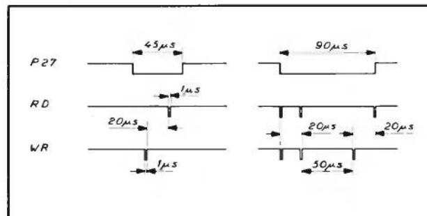
Fig. 2.12 Details of the P27 signal together with the Read and Write signal from the microcomputer.
