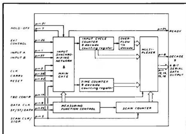
Fig. 2.2 Block diagram of QQ0040.
