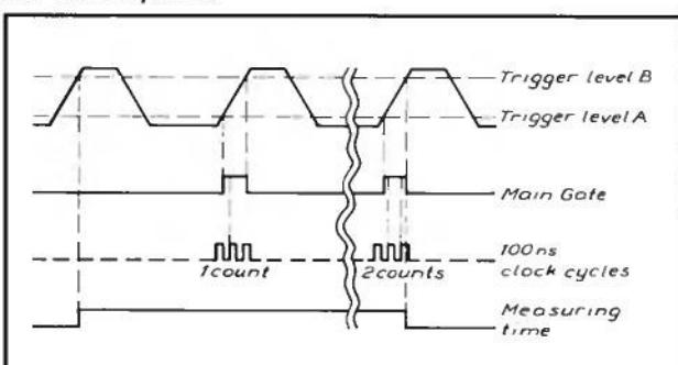
Fig. 2.5 Time Interval Average measurement.
