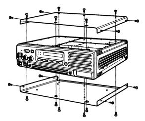
2. Remove cover for RX unit (located in top compartment of repeater).
