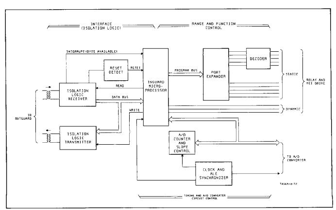
Figure 8-37. Simplified Block Diagram, Inquard Logic.
