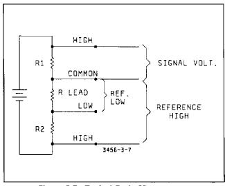
Figure 3-7. Typical Ratio Measurement.
