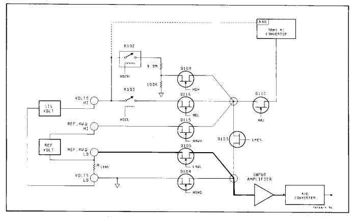
Figure 8-36. Ratio Measurement, Reference Low.
