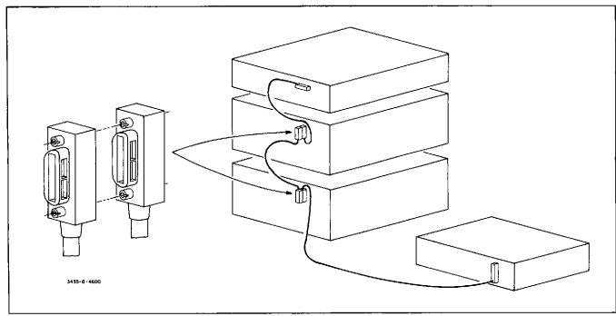
Figure 2-3. Typical HP-IB System Interconnections.
