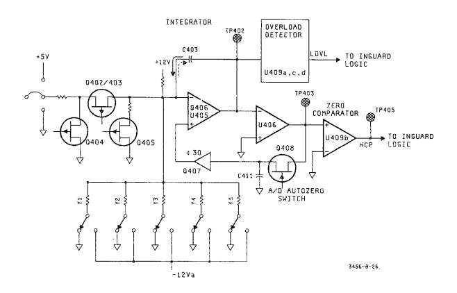
Figure 8-26. Simplified A/D Converter Schematic. 8-19/8-20
