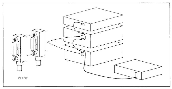
Figure 2-3. Typical HP-IB System Interconnections.
