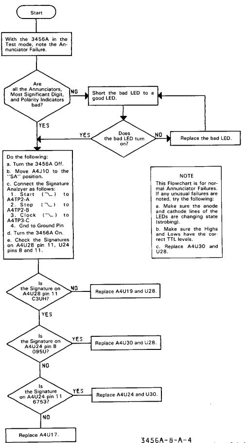
Figure 8-A-4. Flowchart D. Rev B 8-A-9/8-A-10
