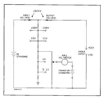
Figure 5-3. DCV Test Equipment Connection
