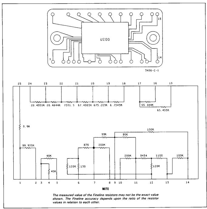
Figure C1. A20U200 Signal Conditioning Fineline (1QD4-0044).
