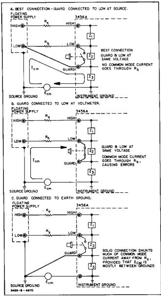
Figure 3-9. Guard Connections.
