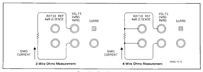
Figure 3-5. Ohms Connection.
