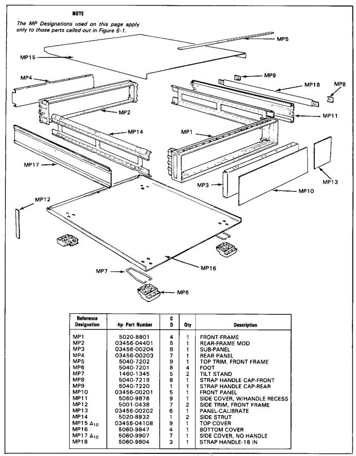
Figure 6-1. Chassis/Cabinet Parts.
