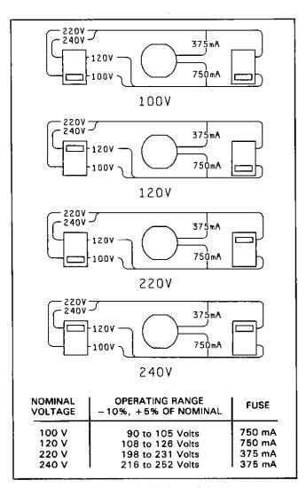
Figure 2-1. Line Voltage Selection.
