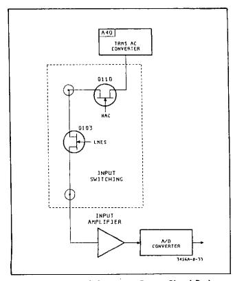
Figure 8-33. AC Converter, Output Signal Path.
