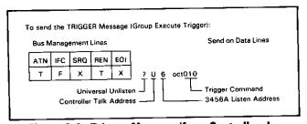
Figure A-4. Trigger Message (from Controller do Device(s)).
