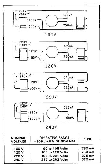
Figure 2-1. Line Voltage Selection.
