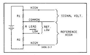
Figure 3-7. Typical Ratio Measurement.
