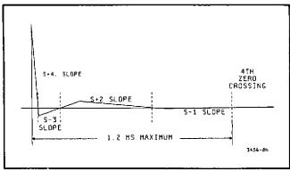
Figure 8-18. Multi-Slope II Rundown.
