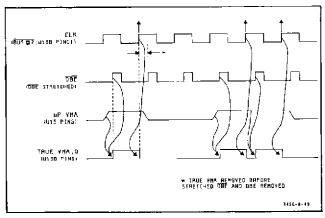
Figure 8-49. True VMA Generator, Timing Diagram.
