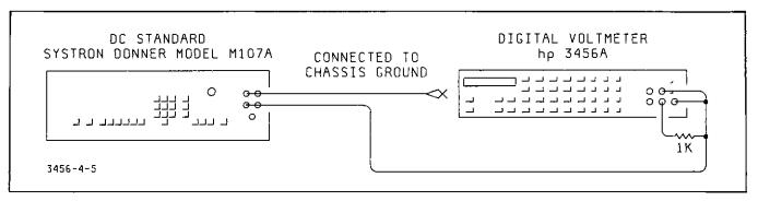
Figure 4-5. DC Common Mode Rejection Test.
