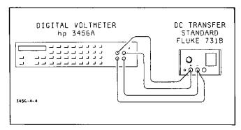
Figure 4-4. Ratio Test Connection.
