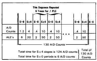
Figure 8-16. Runup Timing Diagram For .1 PLC.
