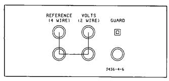
Figure 4-6. 4-Wire Ohms Short.
