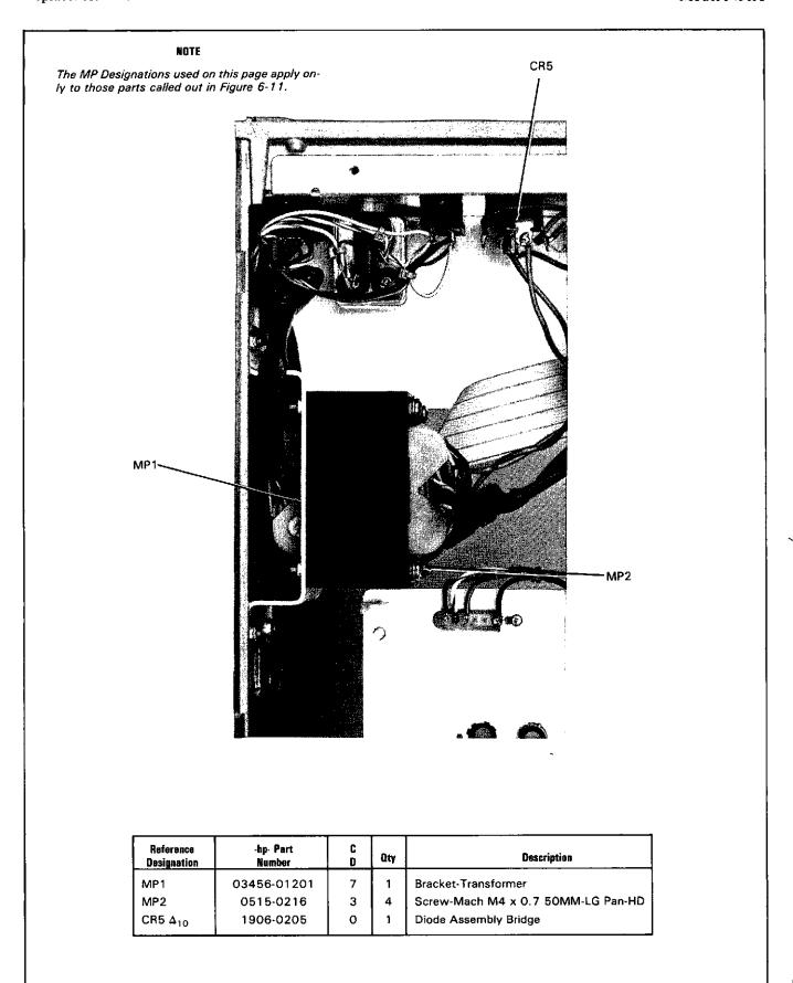
Figure 6-11. Power Transformer and Bracket; Voltage Regulator, Zener Diode, and Bracket.
