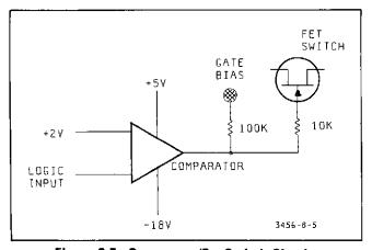
Figure 8-5. Comparator/Fet-Switch Circuit.
