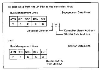
Figure A-3. Data Message (3456A to Controller or Other Device(s).
