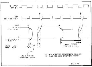
Figure 8-48. Write Going To Read Stretcher, Timing Diagram.
