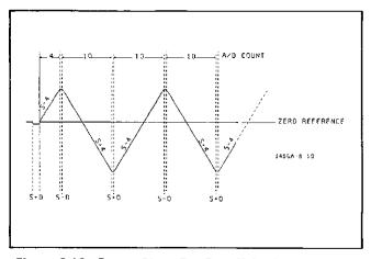
Figure 8-10. Runup Slope For Zero Volts Input (.1 PLC).
