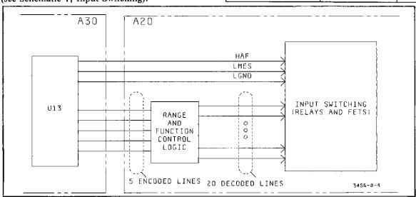
Figure 8-4. Range and Function Control Switching.
