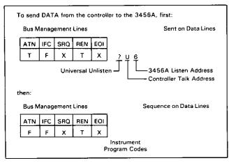
Figure A-2. Data Message (Controller to 3456A).
