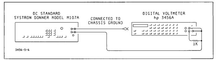
Figure 5-6. DC Common Mode Rejection Test.
