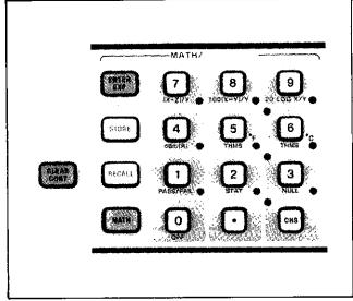
Figure 3-8. Front Panel Numbered Keyboard Area.
