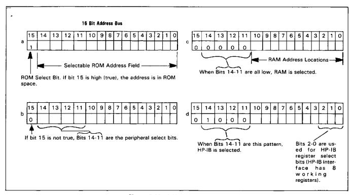
Figure 8-46. Address Bus Structure.
