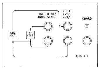
Figure 3-6. Ratio Connection.
