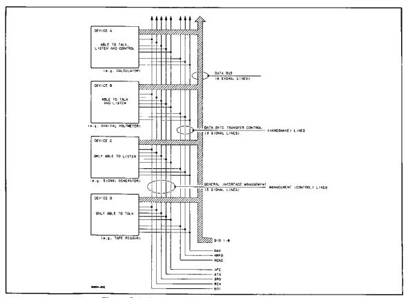
Figure A-1. Interface Connection and Bus Structure.
