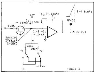
Figure 8-14. Simplified Schematic Of S-4 Slope Generation Circuit.
