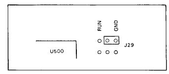
Figure 8-B-1. Test Jumper A20J29 in Ground Position.
