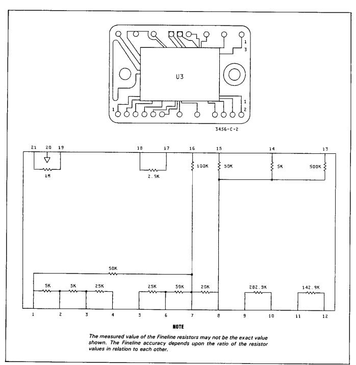
Figure C2. A40U3 AC Gain Fineline (10D6-0046).
