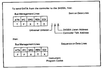
Figure A-2. Data Message (Controller to 3456A).
