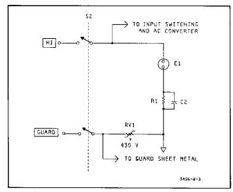
Figure 8-3. High Voltage Protection Circuits.
