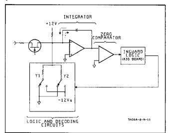
Figure 8-11. Simplified Zero-Crossing Circuit (A/D Converter).
