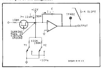
Figure 8-13. Simplified Schematic Of S+4 Slope Generation Circuit.
