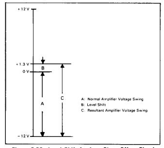
Figure 8-29. Level Shift for Low Ohms Offset Circuit.
