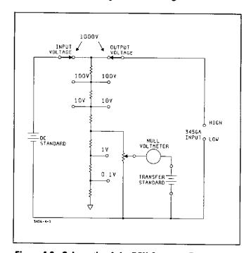
Figure 4-3. Schematic of the DCV Accuracy Test Set-Up.
