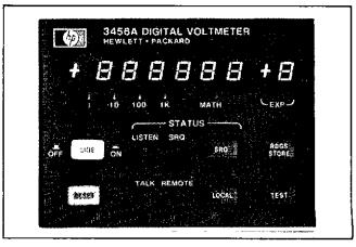
Figure 3-2. Front Panel Display Area.
