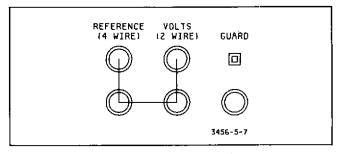
Figure 5-7. 4-Wire Ohms Short.
