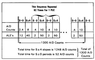
Figure 8-17. Runup Timing Diagram For 1 PLC.
