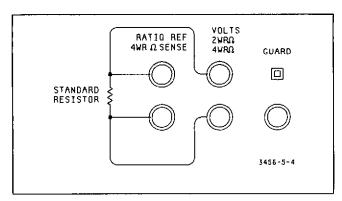
Figure 5-4. Standard Resistor Connection.
