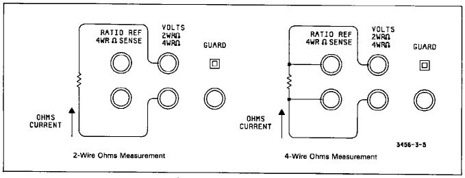
Figure 3-5. Ohms Connection.
