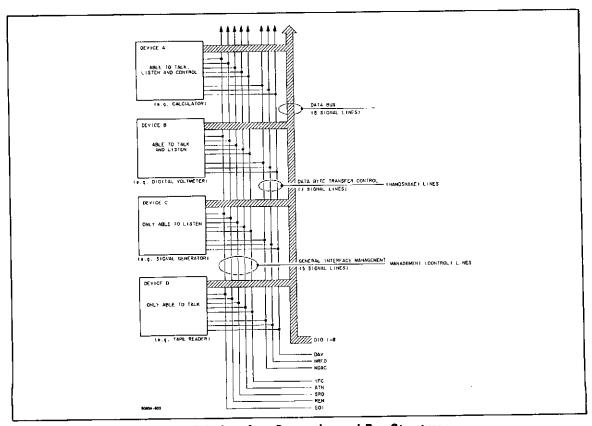
Figure A-1. Interface Connection and Bus Structure.
