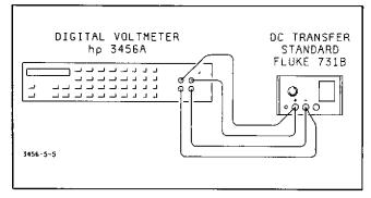
Figure 5-5. Ratio Test Connection.
