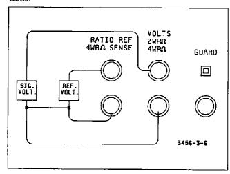
Figure 3-6. Ratio Connection.
