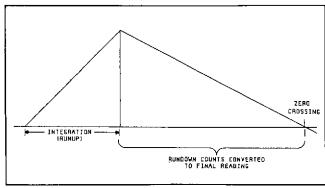
Figure 8-9. Dual-Slope Conversion.
