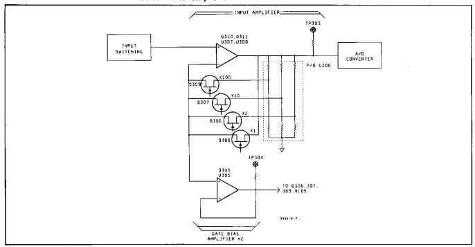
Figure 8-7. Simplified Schematic for Input Amplifier.
