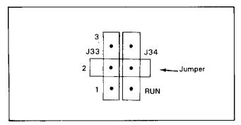
Figure 8-B-2. Jumper A30J33/34 in the 2 Position.
