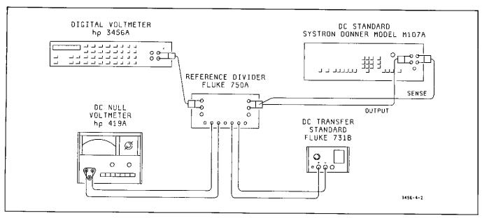
Figure 4-2. DCV Accuracy Test Set-Up.
