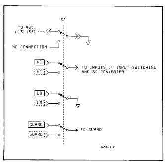
Figure 8-2. Simplfied Front/Rear Switch Circuit.
