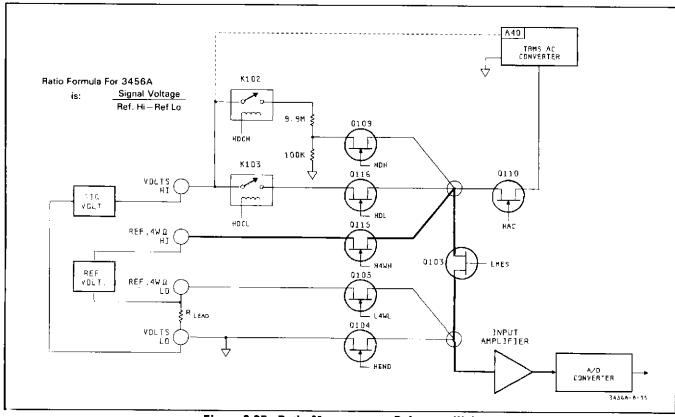
Figure 8-35. Ratio Measurement, Reference High.
