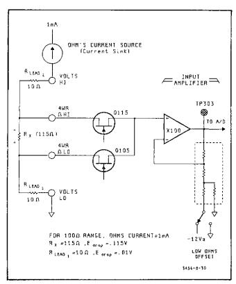
Figure 8-30. Low Ohms Offset, Circuit Operation.
