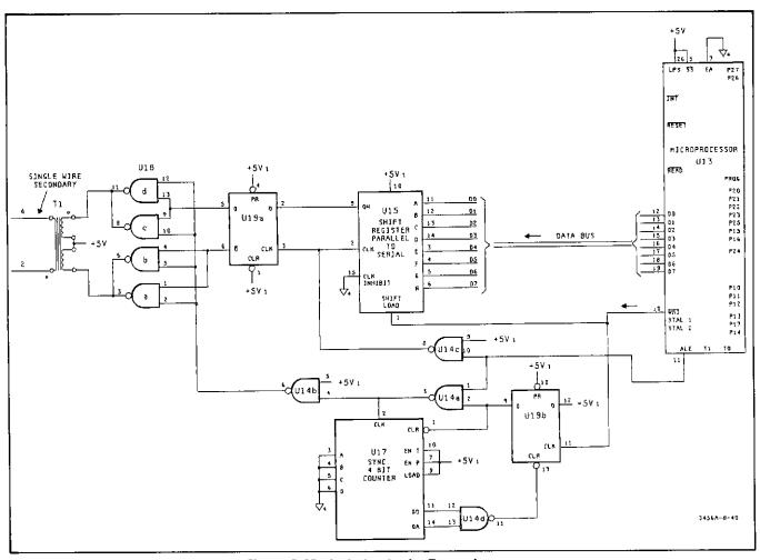
Figure 8-40. Isolation Logic, Transmitter.
