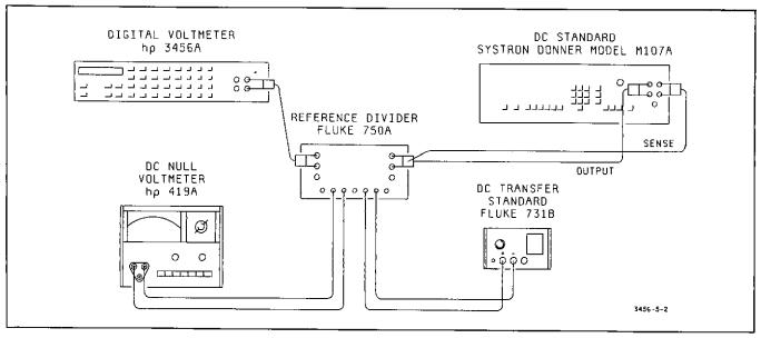
Figure 5-2. DCV Test Equipment Connection.
