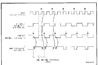
Figure 8-47. DBE Stretcher, Timing Diagram.
