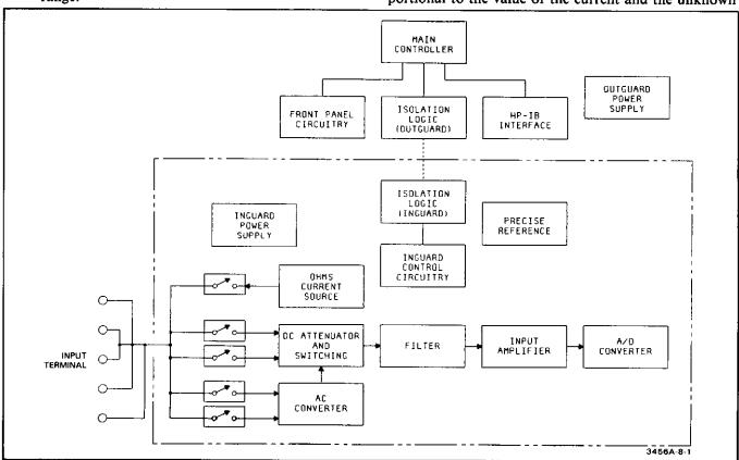
Figure 8-1. Simplified Block Diagram.
