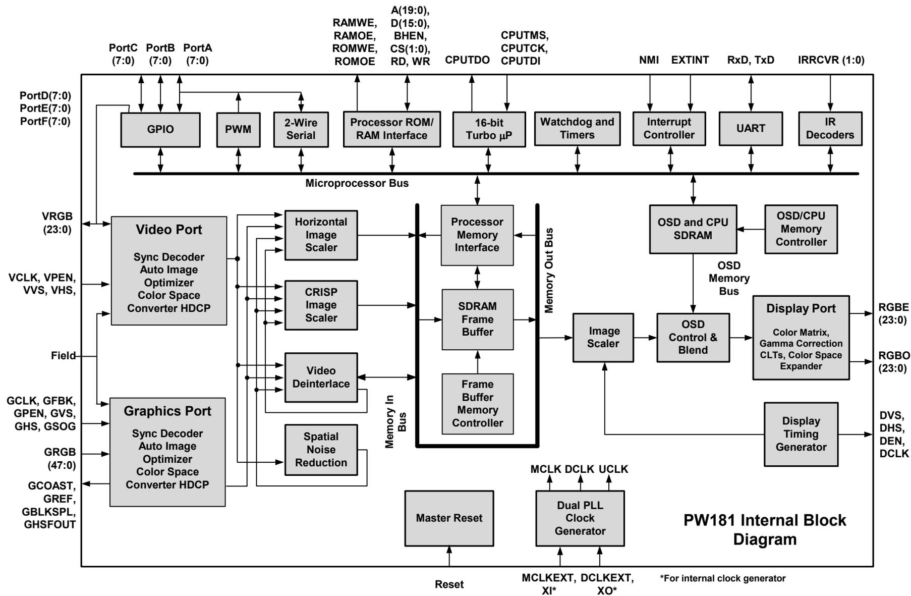
Figure 1-1 Internal Block Diagram
