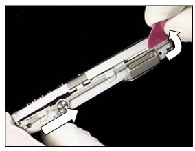
Grip at the bottom then lift *front cover* upwards from the top end of phone.
