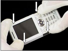
Use **24 Ncm** torque to tighten the four screws with torx bit no. 6.
