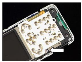
Use the Nylon pointer and insert at the bottom and raise the *PCBA* upwards as shown in picture.
