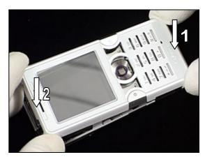
Press down on *front cover* to secure snap hooks as shown in picture.
