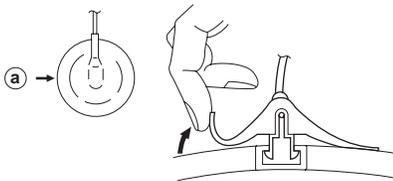
Turn up one side of the rubber cap in the direction indicated by arrow a .
