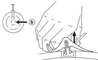
Use your thumb to pull the rubber cap firmly in the direction indicated by arrow b .
