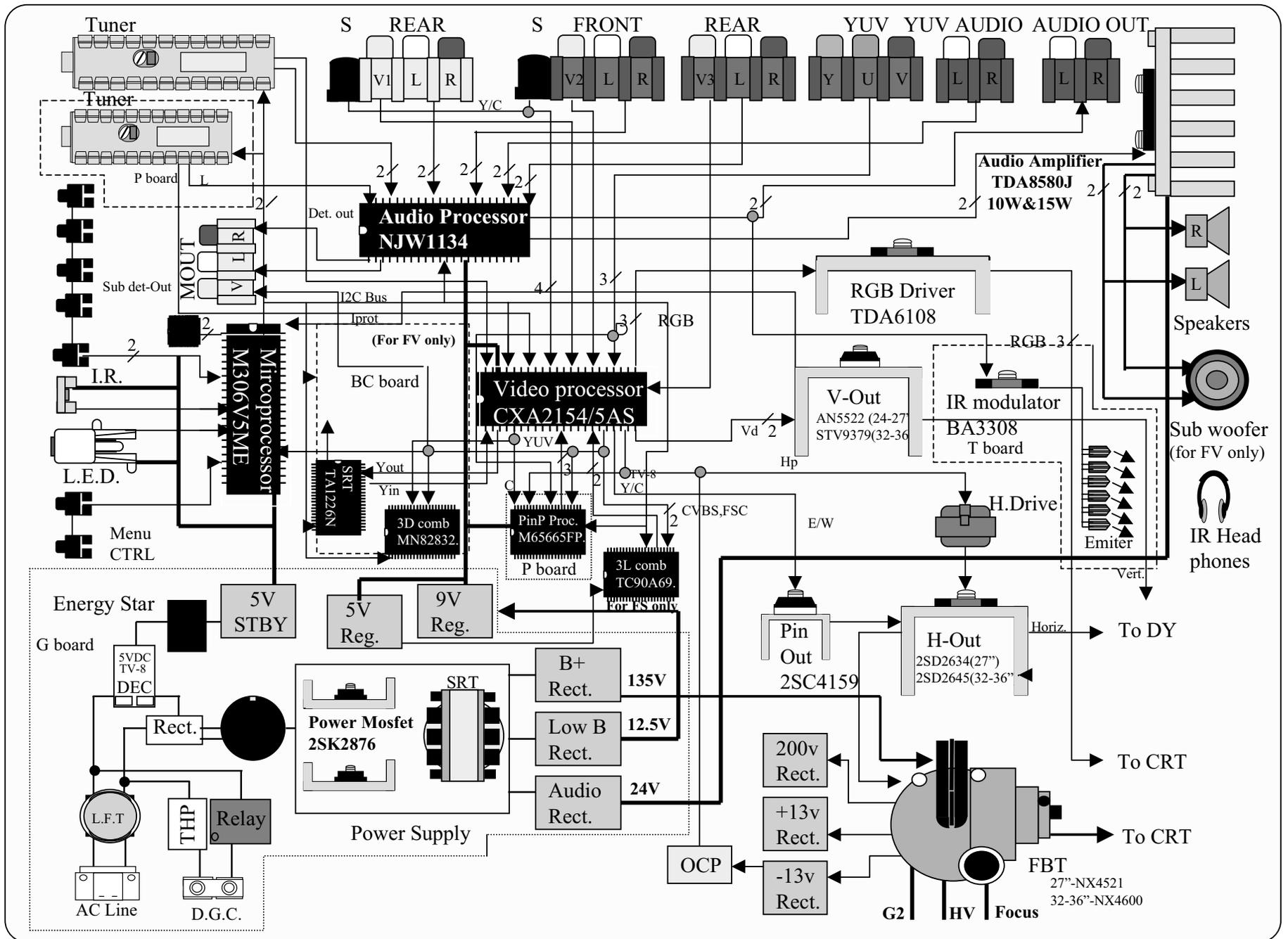
A BOARD SCHEMATIC DIAGRAM
