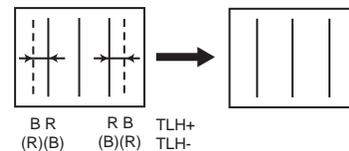
1. Adjust XCV core to balance X axis.
