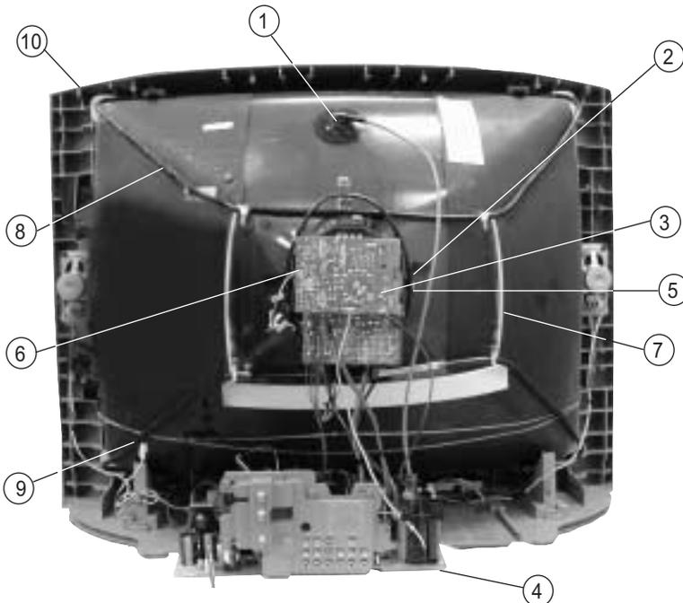
1. Discharge the anode of the CRT and remove the anode cap.
