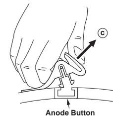
When one side of the rubber cap separates from the anode button, the anode cap can be removed by turning the rubber cap and pulling it in the direction of arrow c .
