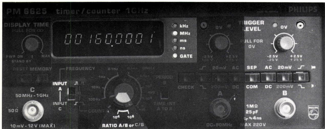
Simple ratio measurement on sine wave and other symmetrical waveforms.
