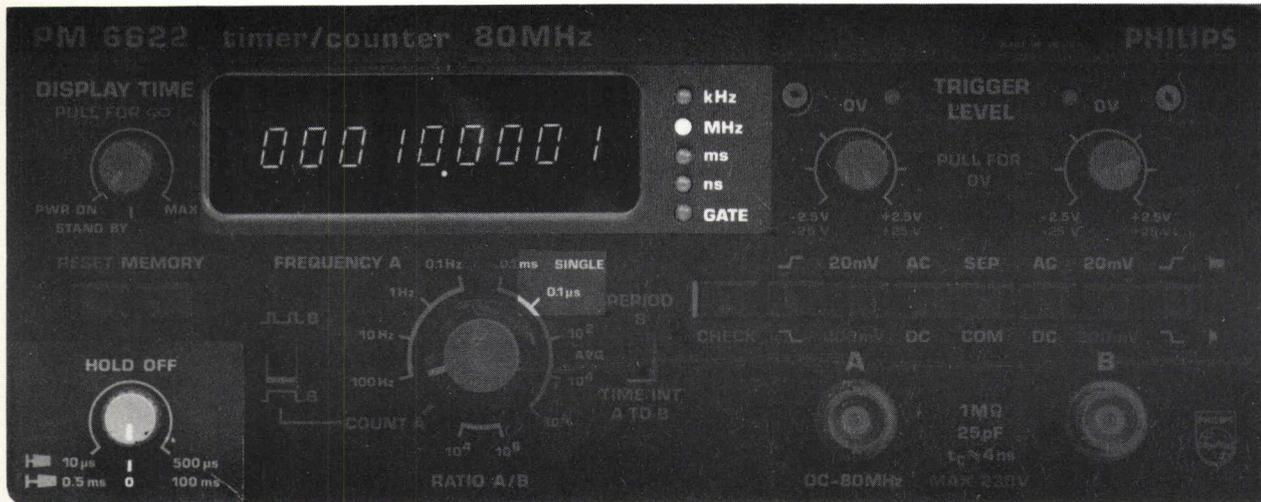
— Set FUNCTION SELECTOR to 0.1  $\mu$ s and rotate HOLD OFF control from fully CCW to fully CW position
