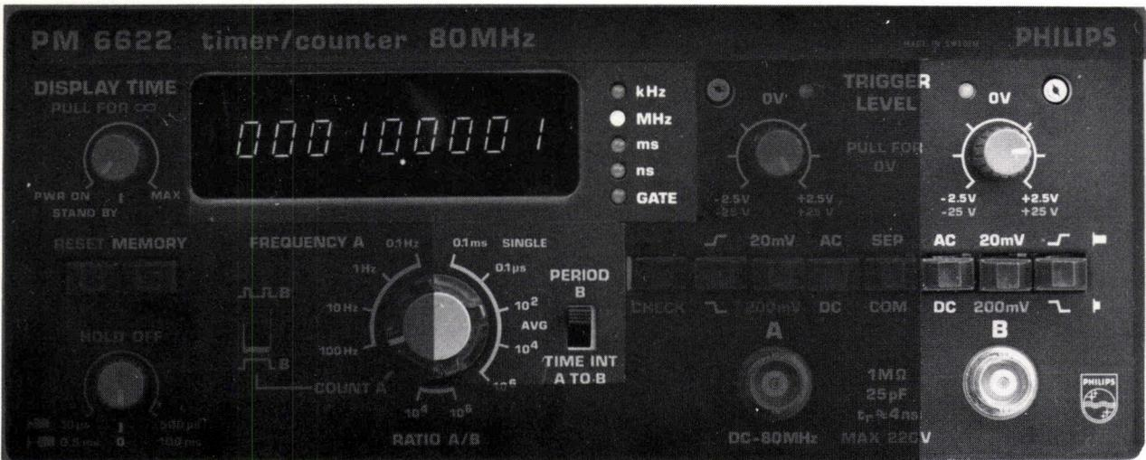
Simple period measurement on sine waves and other symmetrical waveforms.
