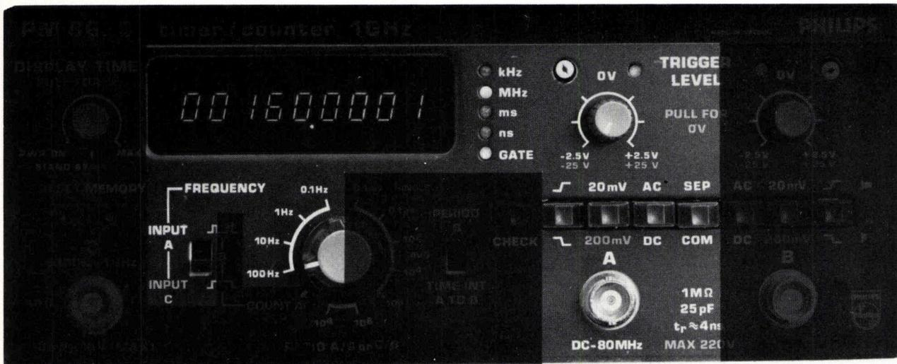
Simple frequency measurement on sine waves and other symmetrical waveforms.
