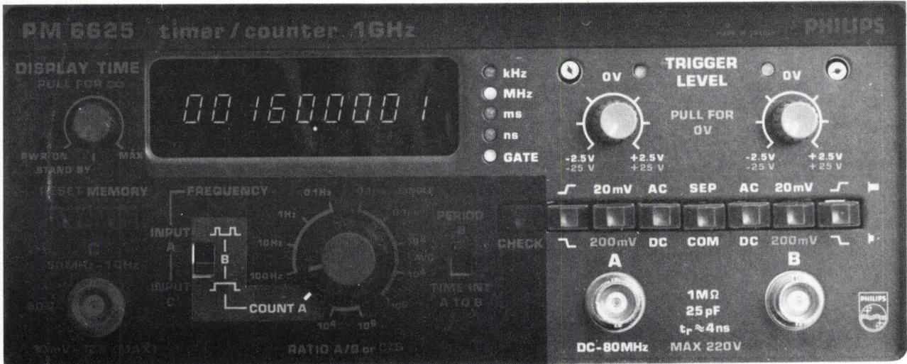
Simple Start/Stop and Gated by B measurement on sine wave and other symmetrical waveforms.
