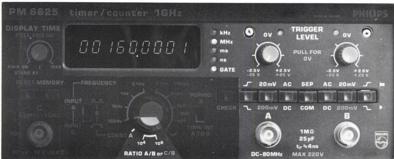
Simple ratio measurement on sine wave or other symmetrical waveforms.
