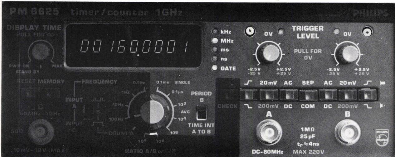
Simple measurement of time interval between pulses at input A and B from separate sources.
