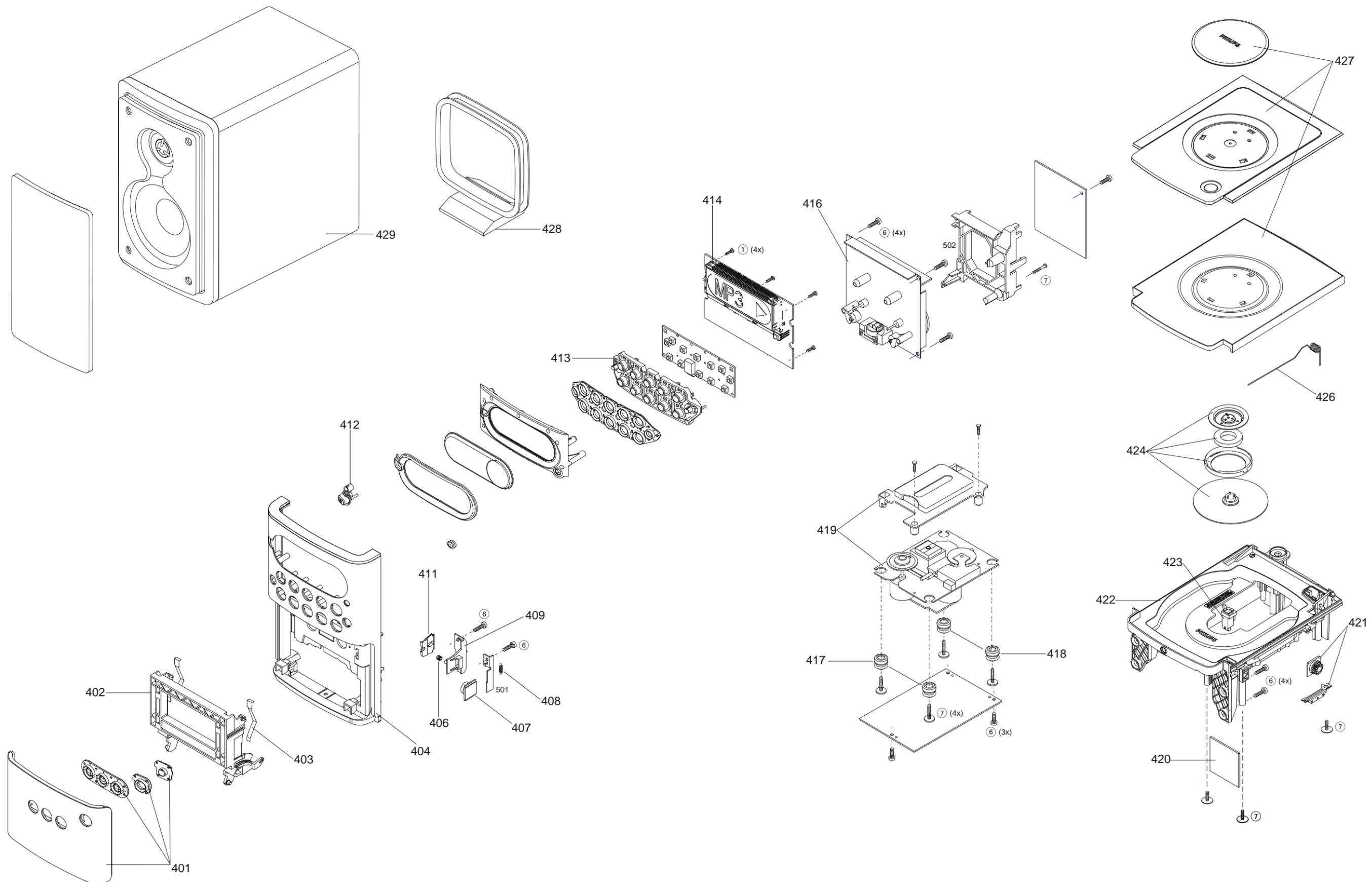
**EXPLODED VIEW DIAGRAM - ETF8 TAPE DECK**
