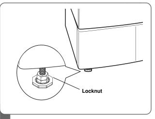
2 Securely tighten all locknuts by hand.
