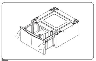
3 Pull up the drawer to disassemble.
