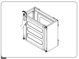
7 Loosen the leg using the wrench.(supplied)
