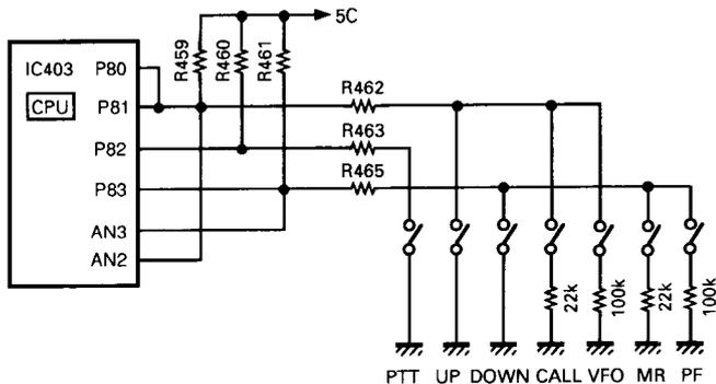
Fig. 14 Microphone key input
