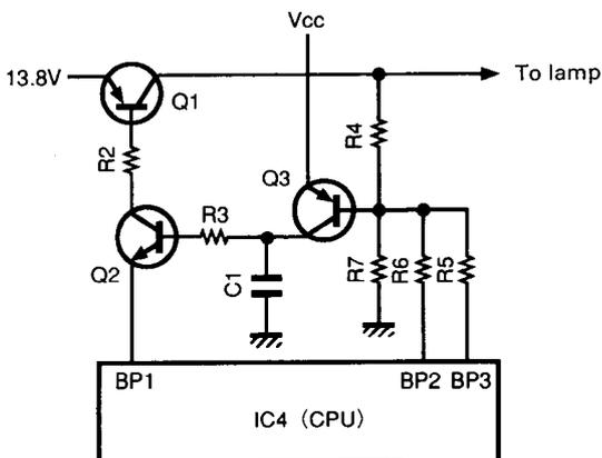
Fig. 15 Dimmer circuit
