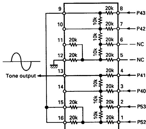
Fig. 9 Internal configuration of ladder resistor
