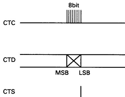
**Fig. 12 Timing chart for CTCSS data transfer**
