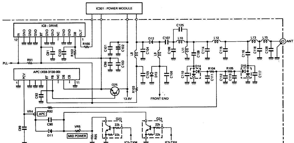
Fig. 3 Pre-amplifier stage, power amplifier, and APC circuits
