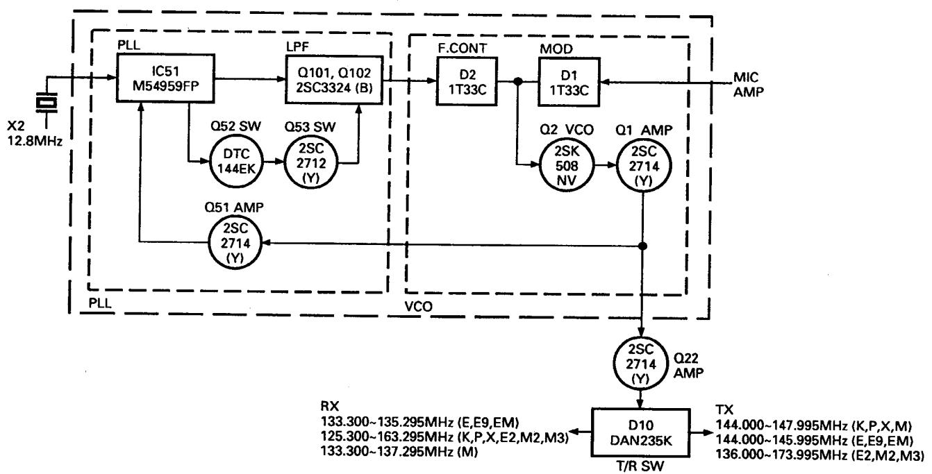
Fig. 4-1 PLL block diagram (K,P,X,M,M2,M3,E,E2,E9,EM)
