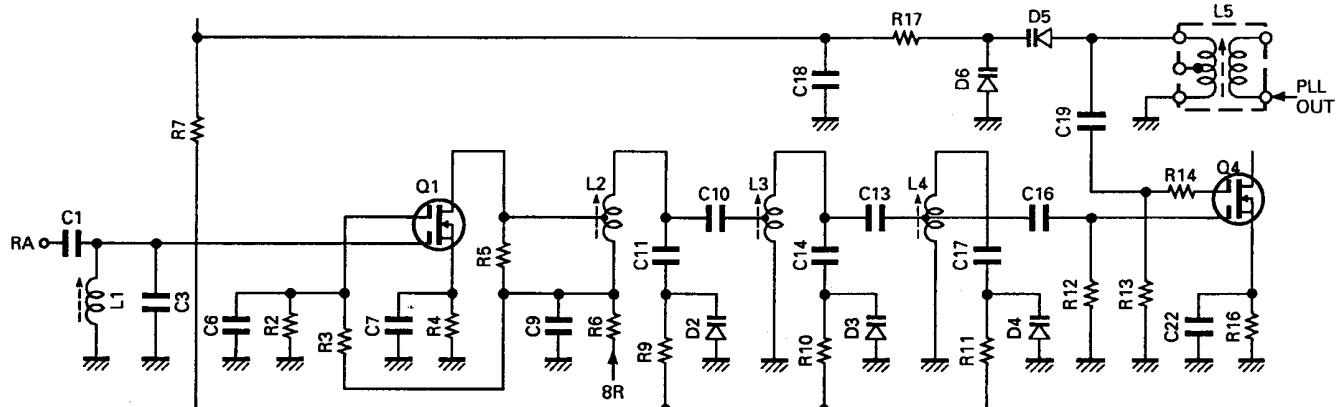
**Fig. 2 Front-end section (vari-cap tuning)**
