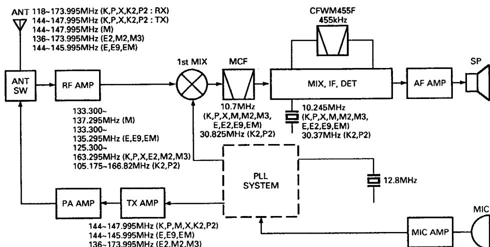
Fig. 1 Frequency configuration
