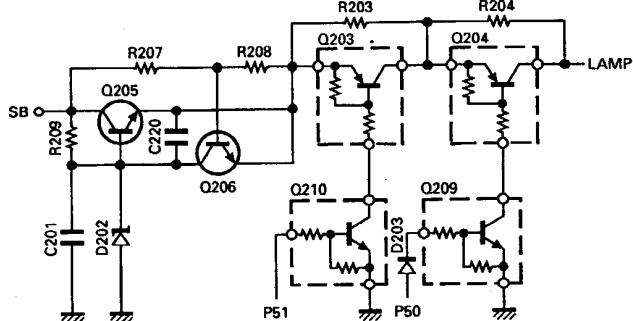
Fig. 8 Dimmer circuit
