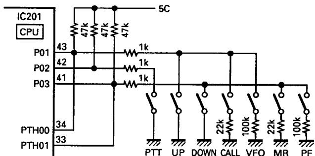
**Fig. 6 Microphone key input circuit**
