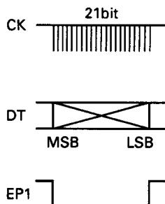
**Fig. 10 Timing chart for PLL data transfer**
