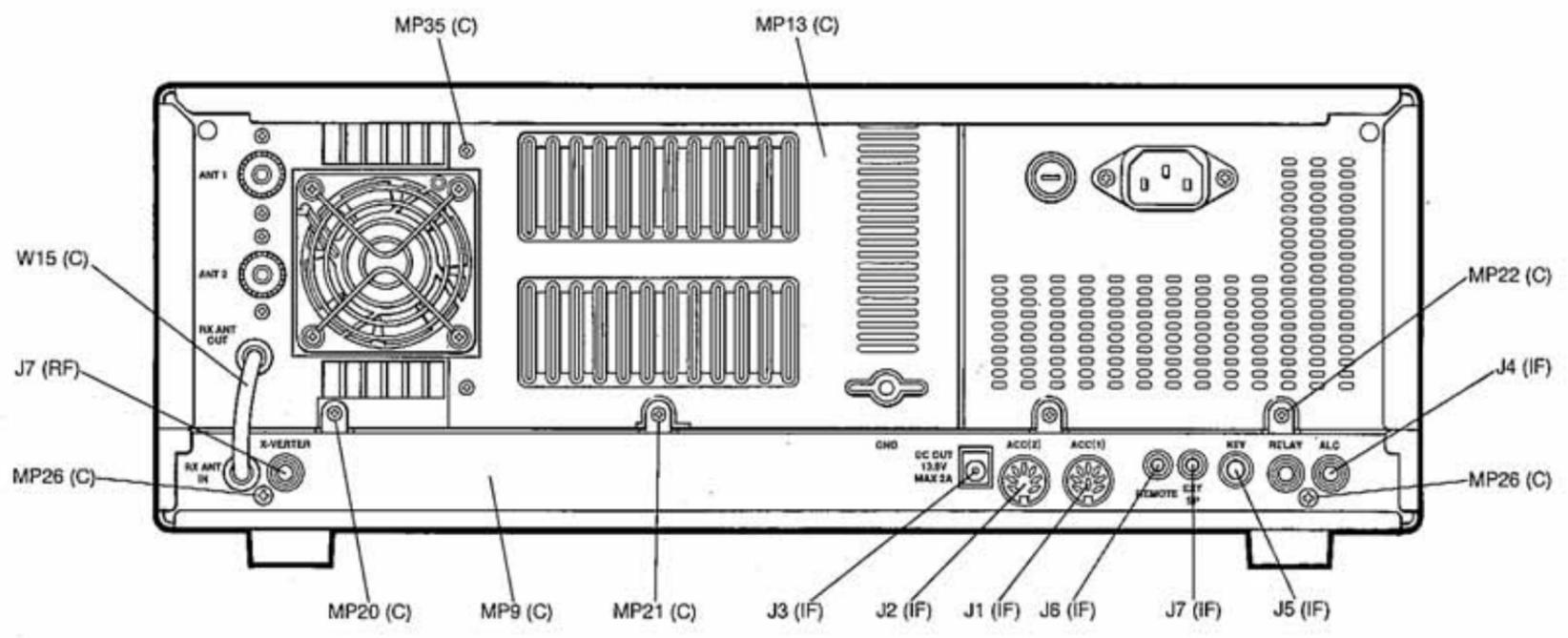
**Unit abbreviations** (C): CHASSIS PARTS (F): FRONT PARTS (J): JACK UNIT (MIC): MIC UNIT (RF): RF UNIT (IF): IF UNIT
