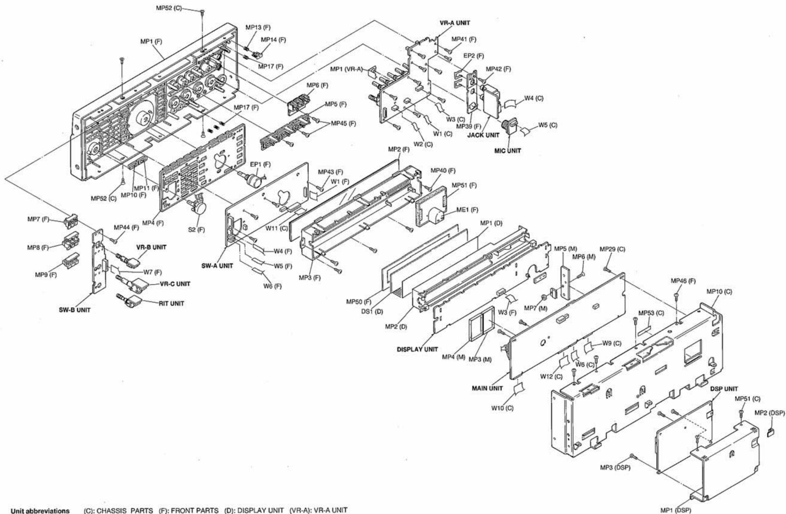
**Unit abbreviations** (C): CHASSIS PARTS (F): FRONT PARTS (D): DISPLAY UNIT (VR-A): VR-A UNIT
