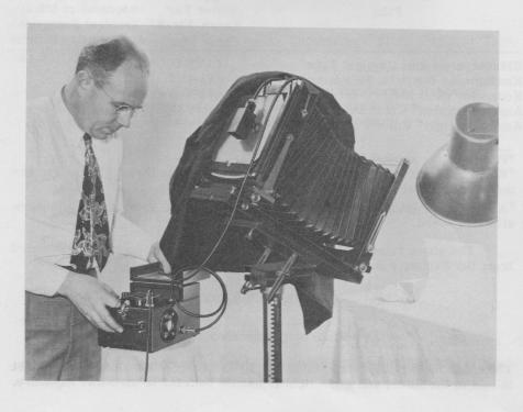
sharp image of card on ground glass. Next, attach probe to ground glass over image of white card, and cover back of camera and probe with black cloth to exclude all external light. Open the lens and press control button to operate flash and note meter reading. The stray light entering the probe from the back can be measured by covering the front of the camera lens so that no light falls on the ground glass from the front.
