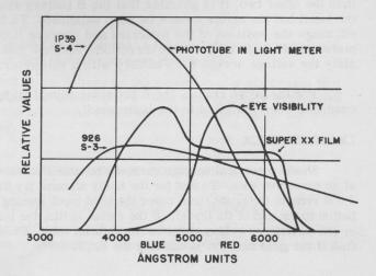
seconds per square foot unless the spectral distribution is the <u>same as the xenon flashtube</u> that is used for calibration. All xenon flashtubes, to a first approximation, have a comparable spectral distribution and therefore the meter readings can be given in terms of lumen-seconds even if the phototube spectral sensitivity does not match that of the standard eye.
