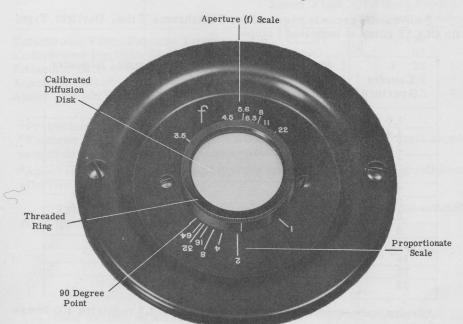
Figure 1b. Close-up of Polaroid Light Attenuator
