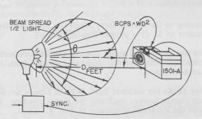
Figure 5. Method of Measuring the Output of a Flash Unit in BCPS. (Beam-Candle-Power Seconds)
