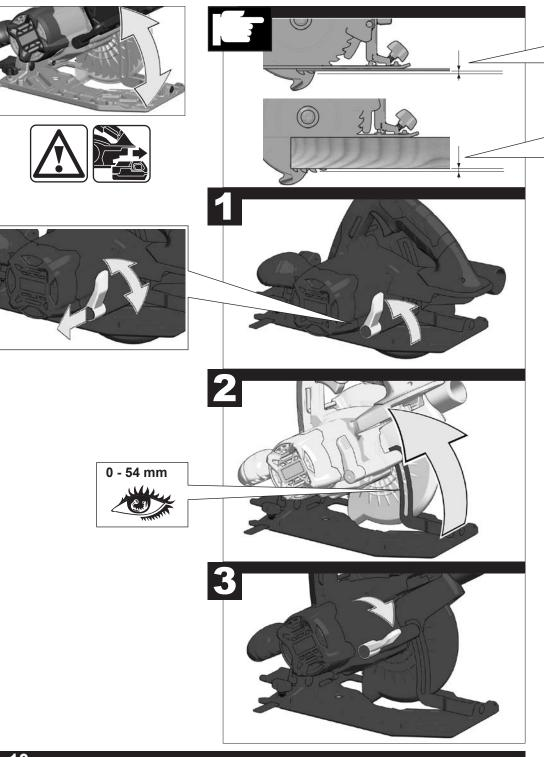
Adjust the cutting depth to the thickness of the workpiece. Less than a full tooth of the blade teeth should be visible below the workpiece.
