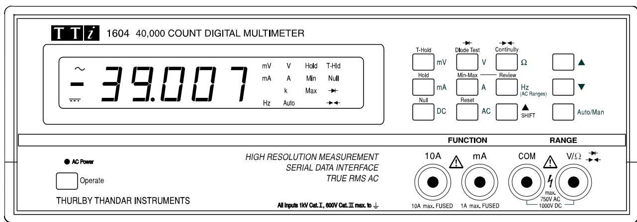
Selection of the primary function is made directly by pressing the appropriate keys e.g. V and DC for DC Volts; the primary function is showing beside the key. The meter is switched between autoranging and manual with alternate presses of the Auto/Man key; alternatively using the arrowed up and down keys changes the range and sets manual ranging.
