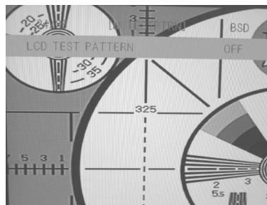
**Fig. 2 Test pattern selection screen**
