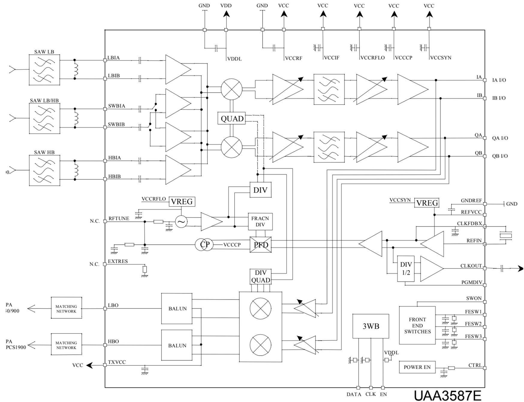
5-2. Base Band Solution Block Diagram
