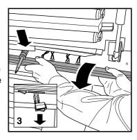
To disassemble the gas pressure springs (50), fold the canopy up and have a second person lock it in this position.
