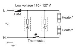
\* Please notice that the upper- and lower heating elements are connected in series. (see electrical diagram). Therefore the voltage and power from one element is the half of the rated voltage and power of the appliance.
