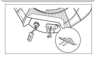
① Loosen the M6 heater nuts to pull out the HEATER ASSEMBLY.
