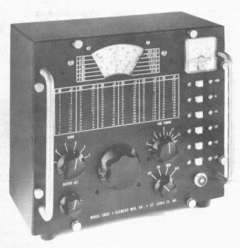
The Model SG-83 Standard Signal Generator is a laboratory test instrument which generates accurately known r-f voltages in the 360 kc to 30 mc range. Either unmodulated or modulated signals may be obtained. This instrument makes possible for the first time at moderate cost accurate laboratory measurements which are essential in communication circuit development and testing.
