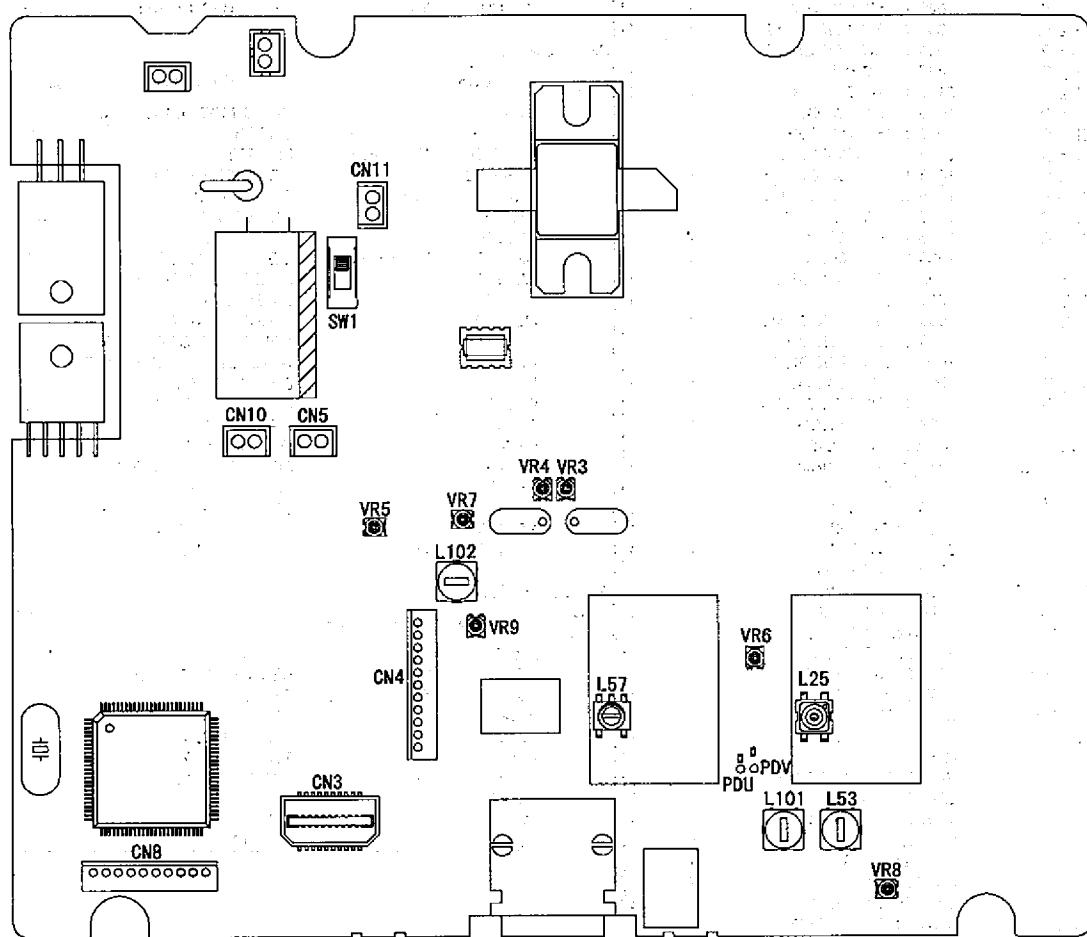
Attention : Don't set the variable resistor into its open position.
