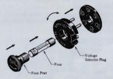
Your machine is equipped with a universal voltage selector offering six selections of voltage from 100V to 240V AC. Voltage is preset at the factory according to destination. However, the operator is requested to reconfirm setting and, if necessary, readjust as follows:
