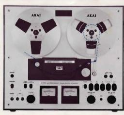
Place a full reel of tape on the Supply Reel Table and an empty reel on the Take-Up Reel Table. Thread the tape as illustrated by the dotted lines in the figure. Lock reels into place with Reel Retainers provided on reel shafts.
