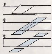
Cut tape diagonally with an overlap so that the ends are lined up (cutting on diagonal eliminates detection of splice in recording). Cover aligned ends with splicing tape. Press firmly exerting pressure to secure ends evenly. Trim off excess splicing tape, cutting into tape very slightly. The eliminates the possibility of a sticky splice. For smooth and easy tape splicing, Akai's portable tape splicer, Model AS-3 is recommended.
