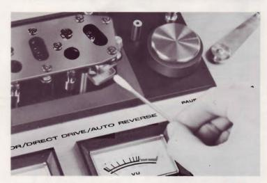
While GX Heads do not require a great deal of cleaning, if old tape which has been spliced, etc. is used, head cleaning is recommended. It is especially important that the heads be clean prior to recording. Remove head cover and clean the heads with a cotton swab stick which has been dipped in Akai Cleaning Fluid (from Head Cleaning Kit HC-500). Also clean the pinch roller, capstan shaft, and tape guides, etc. over which the tape travels.
